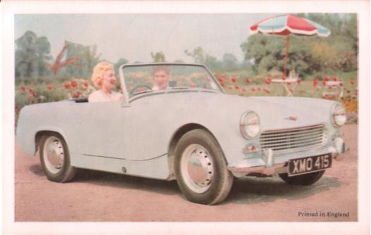
The Austin-Healey Sprite (Mk. II). Twin-carburetter, 'A' Series engine for brilliant acceleration and sportscar performance. Rack and pinion steering, hydraulic brakes, and independent front suspension for safe road-holding. A compact two-seater fully equipped for all-weather motoring.
