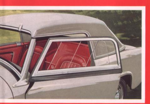
When not in use, the vinyl-treated fabric hood and the metal frame, can be stowed in their hold-all containers in the luggage boot. The quickly detachable, light-alloy frame side-screens have two sliding windows which are easily adjustable for ventilation or hand-signalling. They can be used equally effectively with either hard-top or folding hood.
