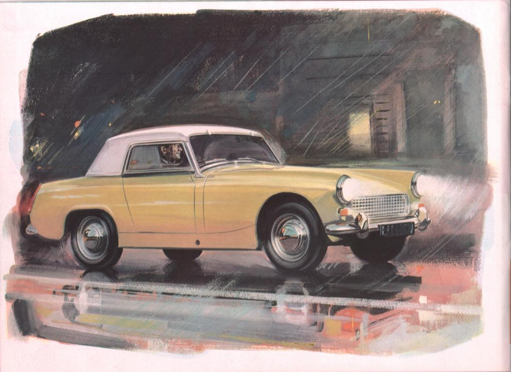
Among the items of optional equipment available is a detachable hard top, which, in effect transforms the Sprite into a comfortable sports saloon. Constructed from tough resin bonded fibre glass, the hard top can be easily removed when the opportunity for open-car motoring prevails.
