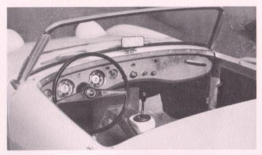
Cockpit layout is remarkably functional with all controls arranged for maximum convenience. Instrument cluster is placed directly in front of driver. Bucket seats upholstered with foam rubber tilt forward to provide access to luggage compartment.
