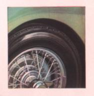
Wire-spoke wheels with "knock-on" hubs are fitted as standard equipment.
