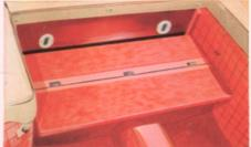
The squab of the occasional rear seats is divided and hinged in such a way that it can be folded forward to form an extended platform 19½ in. (0.49 m.) long and 36½ in. (0.93 m.) wide, when extra space for luggage is required. The surface is covered in the same hard wearing carpet as that of the floor of the car.
