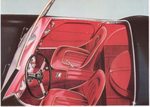
Each of the adjustable bucket seats in the neatly designed interior is upholstered in latex foam rubber with hide facings. On the two seater version the two 6-volt batteries are housed in a locker beneath the spare wheel container. Gears are selected by a short central gear lever and for driving comfort the 17-inch diameter steering wheel has spring spokes. Each door has an open pocket for personal items, and a hard-wearing carpet over the entire floor completes the stylish interior trim.
