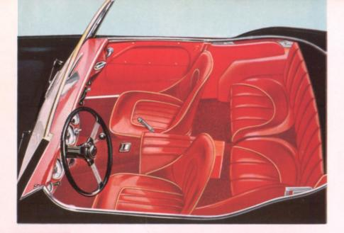
Each of the two front seats is adjustable. The seat cushions are removable and the backs tilt forward to facilitate access to the inset well-type rear seats. An ash tray is provided in the center transmission tunnel. On both two-and four-seater cars a battery master switch operates from inside the luggage compartment, which has a lockable lid, enabling the car to be safely left unattended.
