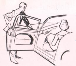
For ease of entry, forward hinged doors open wide and the lower edges lift well clear of the curb or sidewalk. Aluminum framed side screens have one fixed and one sliding plexiglass panel for ventilation or hand signaling.
