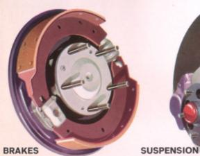
Large diameter hydraulic drum brakes are fitted on the rear wheels and 11½" diameter disc brakes on the front wheels, inspiring confidence at the high speeds of which this car is capable. Sturdy, independent front suspension units and long rear semi-elliptic leaf springs are controlled and stabilized by hydraulic shock absorbers and anti-sway bars.
