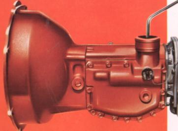
The basic two-or four-seater Austin Healey "3000" Mk.II is equipped with a four speed gearbox which has synchromesh engagement on second, third and top speeds. All components are subjected to rigid scrutiny and testing before assembly to insure maximum efficiency in operation. Power is transmitted to the three quarter floating hypoid rear axle by an open propeller shaft with needle roller universal joints.
