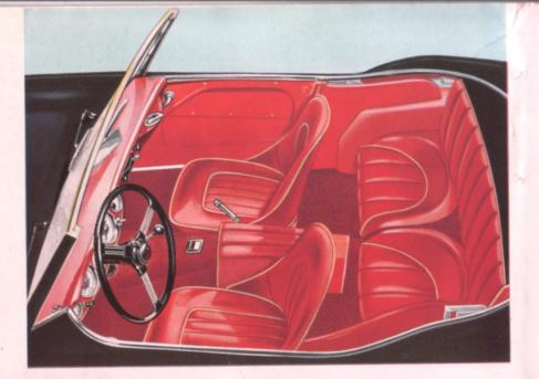
Each of the two front seats is adjustable. The seat cushions are removable and the squabs tilt forward to facilitate access to the inset well-type rear seats. An ash tray is provided in the centre transmission tunnel. On both two- and four-seater cars a master switch operates from inside the luggage compartment, which has a lockable lid, enabling the car to be safely left unattended.
