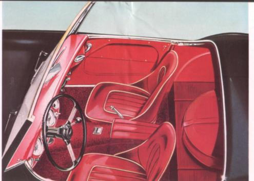
Each of the adjustable bucket seats in the neatly designed interior is upholstered in latex foam rubber, with hide facings. Two 6-volt batteries are contained in a locker beneath the spare wheel container. Gears are selected by a short central gear lever and for driving comfort the 17-inch diameter steering wheel has spring spokes. Each door has an open pocket for personal items, and a hard-wearing carpet over the entire floor completes the stylish interior trim.
