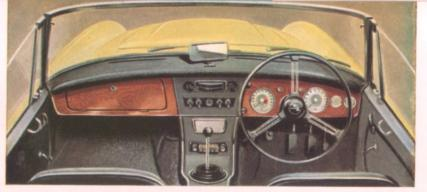
Essential for high-speed travel, the easily read instruments are closely grouped on a wood veneer panel in front of the driver. A short central gear lever in the console permits effortless changes and for driving comfort, the 17 inch diameter steering wheel has spring-spokes. A hard-wearing carpet over the entire floor completes the stylish interior trim. Anchorage points are built-in, to which your Distributor or Dealer can fit B.M.C.-approved accessory seat belts.
