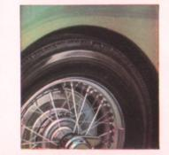
Basic models are fitted with ventilated steel disc wheels, but if continued high speed motoring, or excessive competition driving is intended, then wire-spoke wheels with "knock-on" hubs are strongly recommended It is important that the choice should be made when ordering your car.
