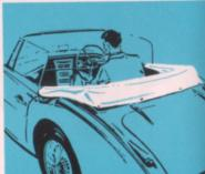
down windows fitted in each door. For increased ventilation the flexible plastic rear window can be un-zipped. When stowed, the hood can be neatly enclosed by a vinyl-coated fabric cover specially tailored for the purpose, so that the Austin Healey 3000 retains to the full, its slick, elegant sports appearance.
