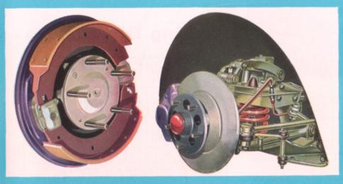
Large diameter hydraulic drum Sturdy, independent front suspension brakes are fitted on the rear wheels and with 11½" (0.29 m.) diameter disc brakes on the front wheels, are servoassisted to inspire confidence at the high speeds of which this car is
