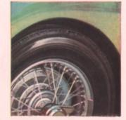
Basic models are fitted with ventilated steel disc wheels, but if continued high speed motoring, or excessive competition driving is intended, then wire-spoke wheels with "knock-on" hubs are strongly recommended. It is important that the choice should be made when ordering your car.
