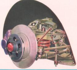
Large diameter hydraulic drum Sturdy, independent front suspension brakes are fitted on the rear wheels and with 111 (0.29 m.) diameter disc brakes on the front wheels, are servoassisted to inspire confidence at the high speeds of which this car is capable.
