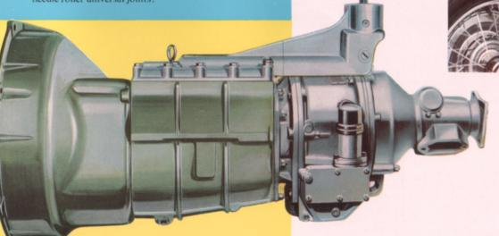
An electrically controlled overdrive (illustrated here) can, if required, be fitted to the standard gearbox of the Austin Healey 3000. This is operated by a switch on the fascia and provides a high top gear ratio giving the car a fast cruising speed, while maintaining a modest fuel consumption.
