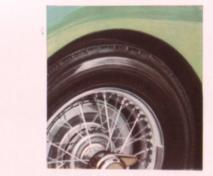
Basic models are fitted with ventilated steel disc wheels, but if continued high speed motoring, or excessive competition driving is intended, then wire-spoke wheels with "knock-on" hubs are strongly recommended. It is important that the choice should be made when ordering your car.
