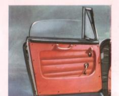
Saloon car comfort when it's needed, and yet, all the thrill of open sports car motoring is available in an instant. Regardless of whether the door windows are raised or not, the tough, vinyl-treated fabric hood can be quickly folded away behind the occasional rear seats. Retained in two places on the screen head-rail, it is but a simple operation to unfasten the quick-release catches and lower the hood.
