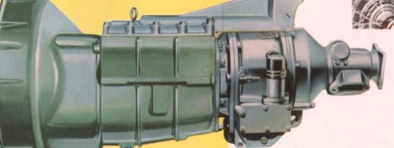
An electrically controlled overdrive (illustrated here) can, if required, be fitted to the standard gearbox of the Austin Healey 3000. This is operated by a switch on the fascia and provides a high top gear ratio giving the car a fast cruising speed, while maintaining a modest fuel consumption.
