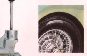
Basic models are fitted with ventilated steel disc wheels, but if continued high speed motoring, or excessive competition driving is intended, then wire-spoke wheels with "knock-on" hubs are strongly recommended. It is important that the choice should be made when ordering your car.
