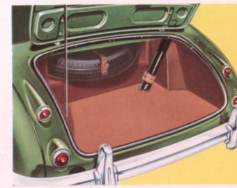
The spare wheel is stowed in a special container in the rear compartment leaving a surprising amount of space available for family luggage. Lighting equipment consists of powerful double-dipping headlamps, flashing direction indicators combined with sidelamps at front and stop/tail lamps at rear. A number plate illumination lamp is mounted in the rear bumper.
