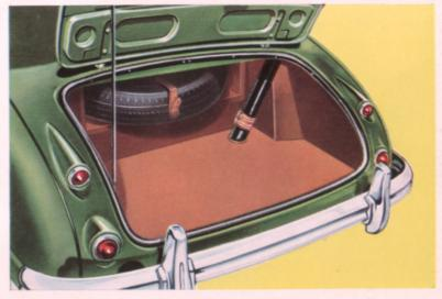
The spare wheel is stowed in a special container in the rear compartment leaving a surprising amount of space available for family luggage. A master switch operates from inside the compartment, which has a lockable lid enabling the car to be safely left unattended.
