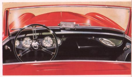
All instruments are easily readable, being closely grouped in a panel in front of the driver. On the opposite side of the trimmed fascia is a grab-handle for the convenience of the passenger.
