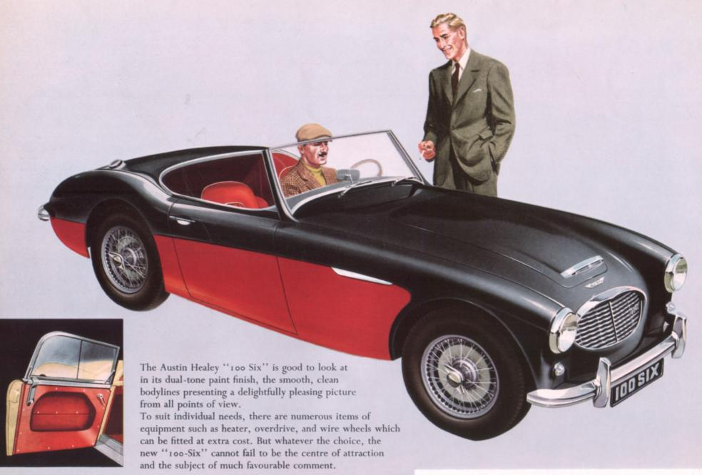
Aluminium framed side screens have one fixed and one sliding perspex panel for ventilation or hand signalling. Anstin Healen
