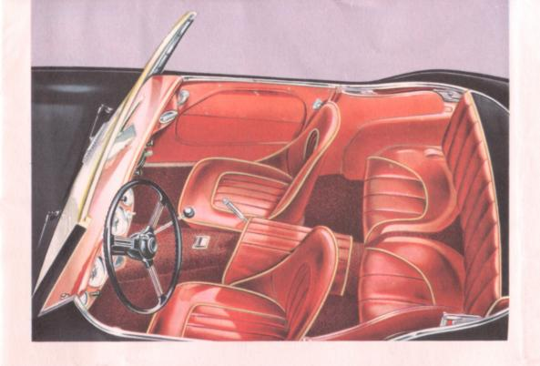
Each of the adjustable bucket seats in the neatly designed interior is upholstered in latex foam rubber, with hide facings. The backs tilt forward to give access to the rear seats.
