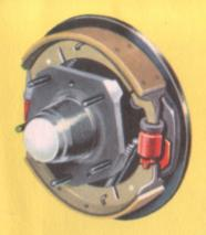
Large diameter hydraulic brakes with two-leading-shoe action on the front wheels ensure powerful and progressive retardation.
