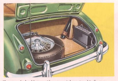
The spare wheel and battery with master switch are stowed in the rear compartment and there is a surprising amount of space available for family luggage.
