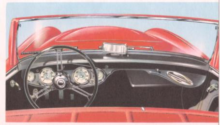
All instruments are easily readable, being closely grouped in a panel in front of the driver. On the opposite side of the covered fascia is a grab-handle for the convenience of the passenger.
