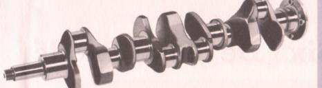
The robust, four-bearing, fully-balanced crankshaft.
