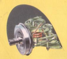
Sturdy, independent front suspension units are controlled by hydraulic shock absorbers and stabilizing bar.
