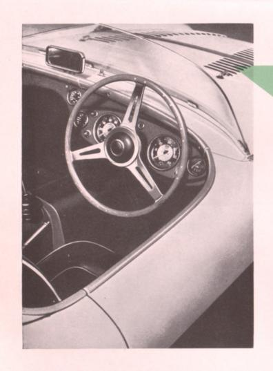
Instrument layout, and duralumin steering wheel with laminated wood rim
