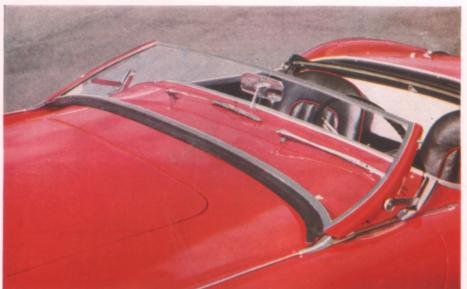
The windshield has two operative positions; raised, for normal driving conditions and lowered to form a scuttle when high speeds are anticipated. The change-over is readily effected and a positive locking device ensures absolute security in either position. The illustration (left) shows the windshield neatly lowered and enclosing such protrusions as windshield wipers and driving mirror.
