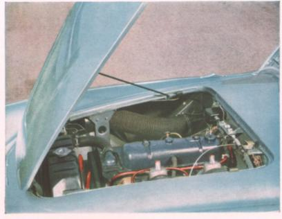
The hood is hinged along its forward edge and opens widely to give good access to the engine and ancillary components for routine maintenance.
