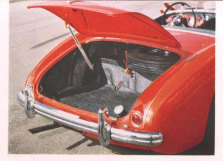
An exceptionally spacious luggage compartment for this type of car is provided at the rear. It also accommodates the spare wheel in a separate recessed shelf and encloses the fuel filler pipe.
