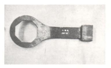
This heavy duty wrench has been designed for workshop use. Made out of 1/4" high grade steel plate - handle angled and reinforced with 3/4" lug. Fits all BMC models with hexagonal knockoffs.
