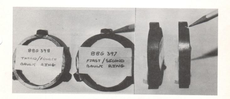
The same identification is used on the MGC transmission with a part number change for the third/fourth baulk ring.
